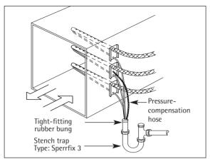
Because of the under-pressure in the appliance or the duct part, condensate may be kept back in the steam-distribution pipe. If there is an outlet in the empty part of the humidifier, the condensate can be bled off in the immediate vicinity. An alternative method of bleeding off the condensate can be seen in the diagram.
